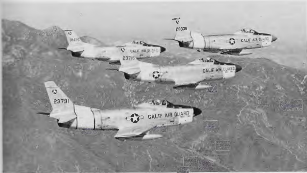
Left: NORTH AMERICAN F-86D "SABRE." In March 1958, after the formation of the 163rd Fighter Group (Air Defense), a new F-86 model arrived at Ontario. The F-86D, more often referred to as the "Dog," provided the squadron with its first all weather capability. This air interceptor version of the F-86 carried no guns. Instead, it was equipped with the Hughes E-4 fire control system and armed with 24 2.75 inch rockets. This lethal punch could destroy any known manned bomber, and the aircraft could find and kill its target in any kind of weather.
