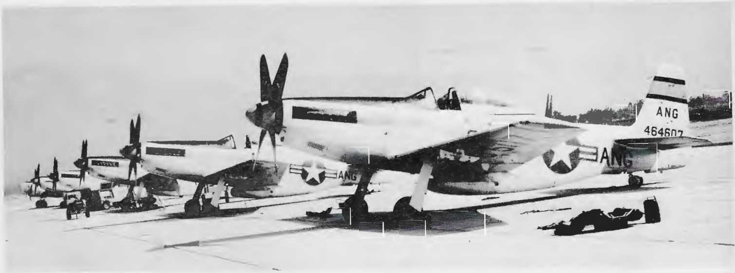
Above: NORTH AMERICAN F-51H "MUSTANG." In Oct., 1952, after the 196th Fighter Squadron was released from active duty, the unit was reassigned propeller driven aircraft. The uprated H model of the Mustang was the most powerful of the series. This is the first aircraft assigned to the Ontario ANG base.
