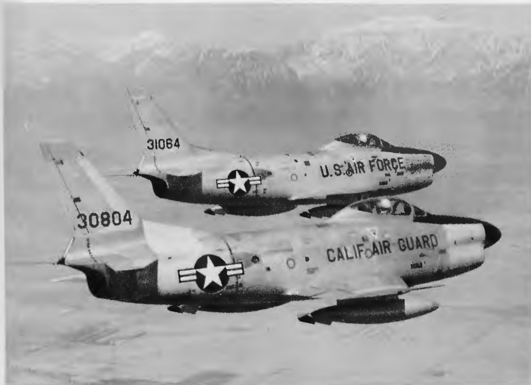
Left: NORTH AMERICAN F-86L "SABRE." In Feb., 1961, the 163rd Fighter Group (Air Defense) traded in its F-86D aircraft for F-86L's. This aircraft, although it looks much like the F-86D, contained many improvements. Some of the modifications included changes in cockpit instrumentation, and a lengthened wing. The group flew this aircraft from 1961 to 1965, when it received the first of its F-102 "Delta Daggers."
