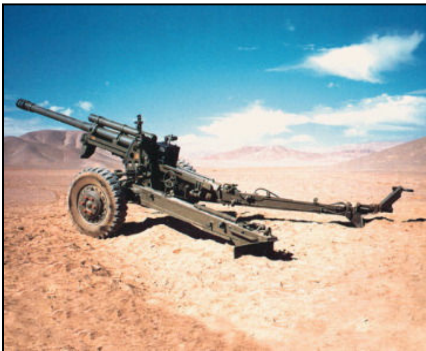
The M101A1 105mm Light Howitzer. Source: National Archives The basic light artillery weapon of World War II and Korea. Towed behind a 2 ½ ton 6x6 truck. It was used for both direct and indirect fire.
