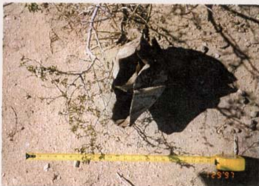
J-8 Area A: M38A2 100 lb practice bomb tail fin assembly at western edge of dry lake; see plate 4.
