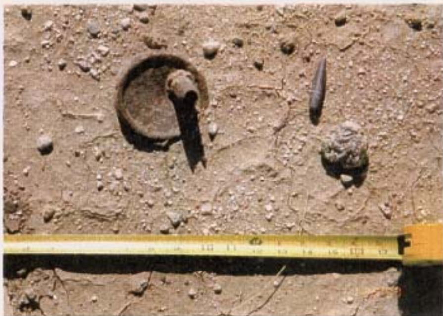
J-4 Area A: M1A1 spotting charge debris and .50 cal projo southwest of target center; see plate 4.
