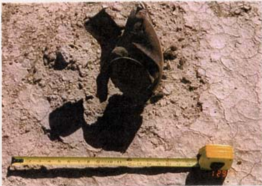
J-1 Area A: Debris from M38A2 100 lb practice bomb near target center; see plate 4.
