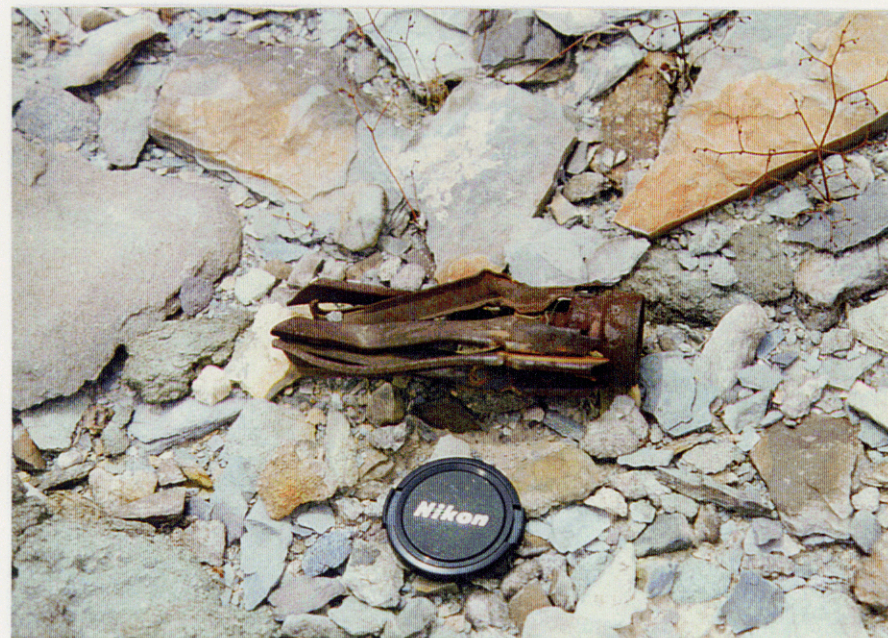
J-10 Fins from a 2.36 inch Rocket found on the Bunker Assault Range
