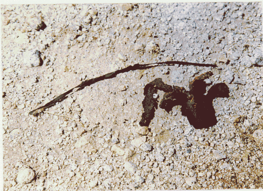
J-23 81MM mortar debris and fragment from a large caliber artillery projectile on LFR
