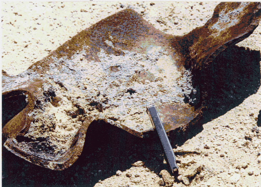
J-17 Close-up of thick case bomb with residual concrete filler
