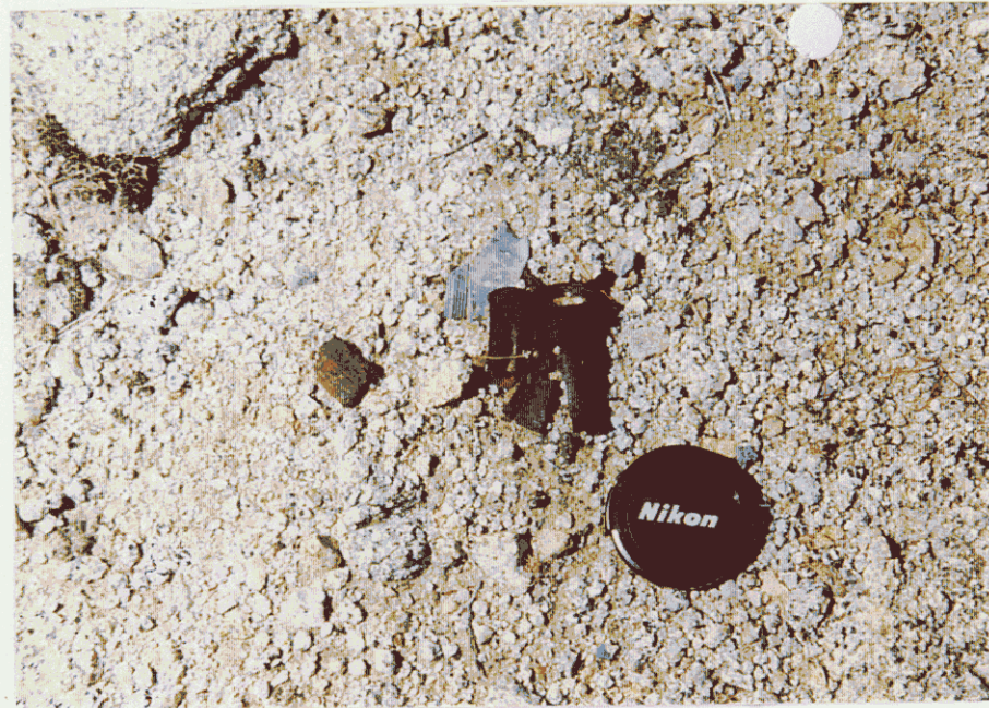
J-22 Sample of 60MM mortar debris uncovered on LFR
