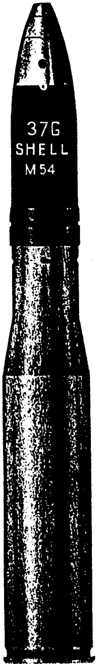
Figure 33 - SHELL, Fixed, H.E., M54, w/TRACER, SD, and FUZE, P.D., M56, 37-mm Auto. Guns, M1A2 and AN-M9
