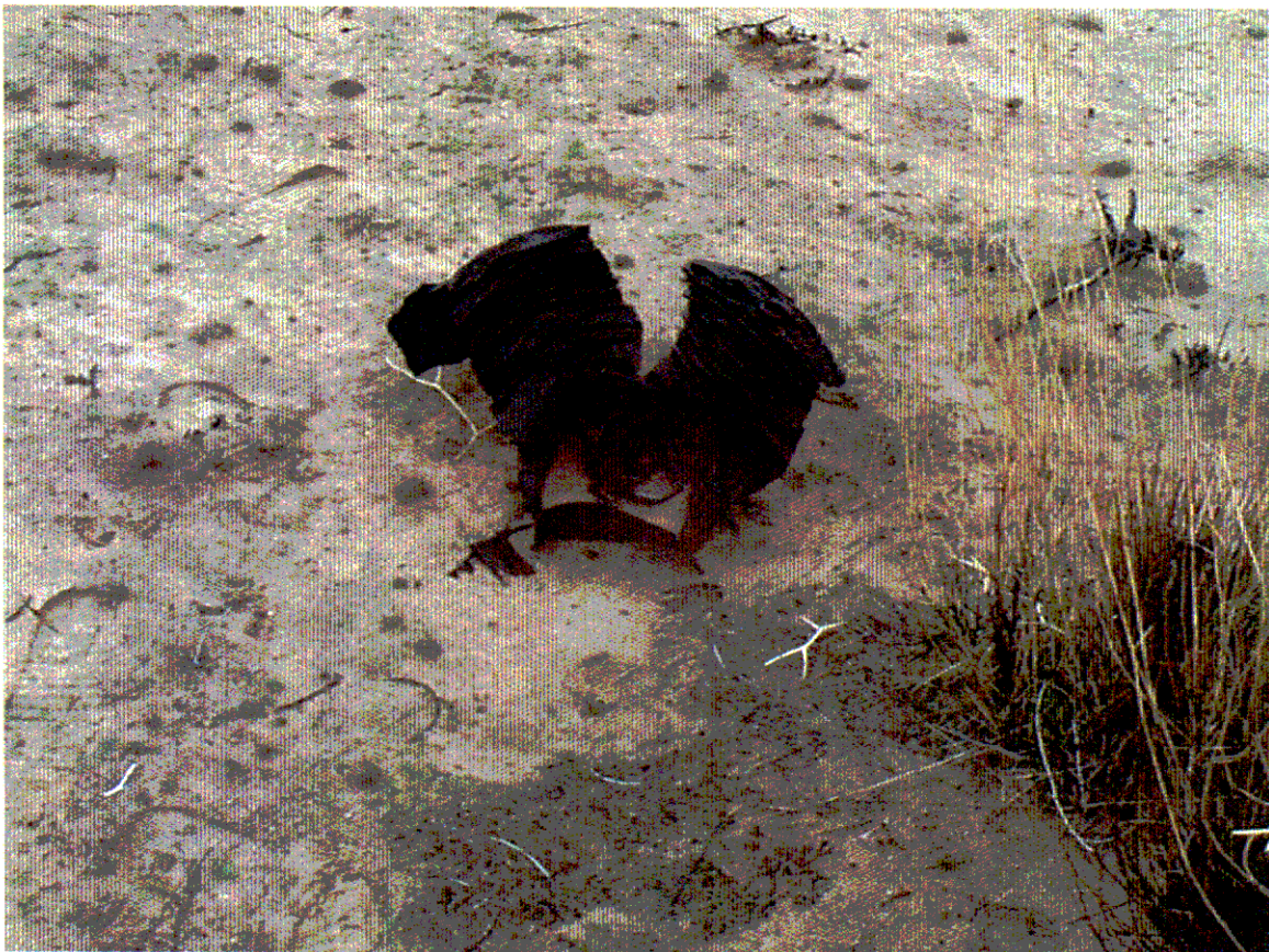
J-2 Tail Fin Attached to Bomb Body (Area A: Impact Area)
