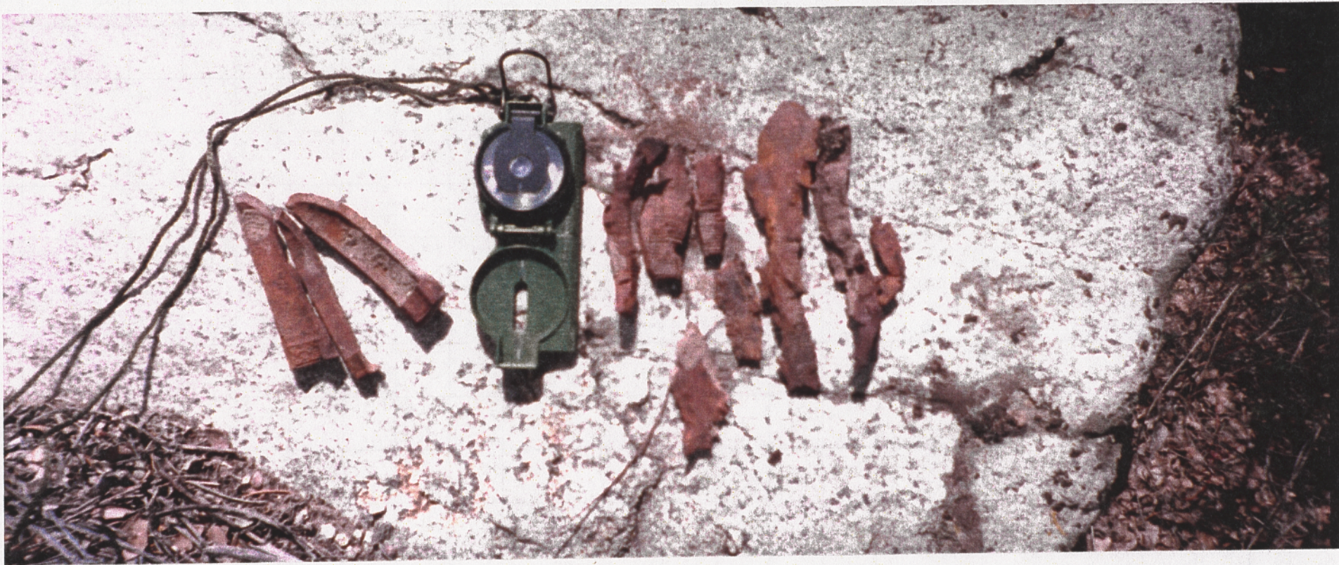
J-5 Shrapnel from 37mm ammunition and 105mm ammunition that was being found during this inspection in Areas A.
