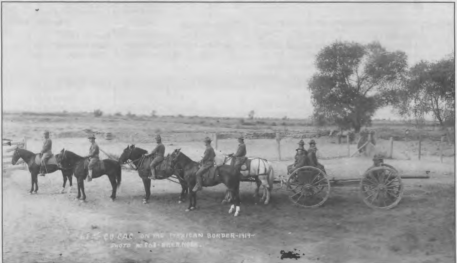
Figure 15: U.S. Model 1897 3.2 inch field gun (right) with attached ammunition limber in use by the 61st Coast Artillery Company from Fort Baker, at Calexico, California. Such limbers, detached from their cannon, were used to move explosives around San Francisco during the 1906 fire, but the cannons themselves were never used. Caissons, or large limbers without the provision for cannon attachment, were likewise employed. Eight years later, First Sergeant Dillon and his elite unit was sent to the Mexican Border (marked by the fence in the background) as a response to revolutionary turmoil south of "the line." Partial enlargement of panoramic shot by G. R. Nock, late April or early May, 1914. Dillon Collection.
