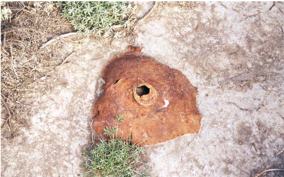
Photo #2 - Siskiyou Rocket and Bombing Range – 27-31 August 2001 OE Debris 100-lb. Practice Bomb – nose and filling plug portion of Navy MK VII or XV.
