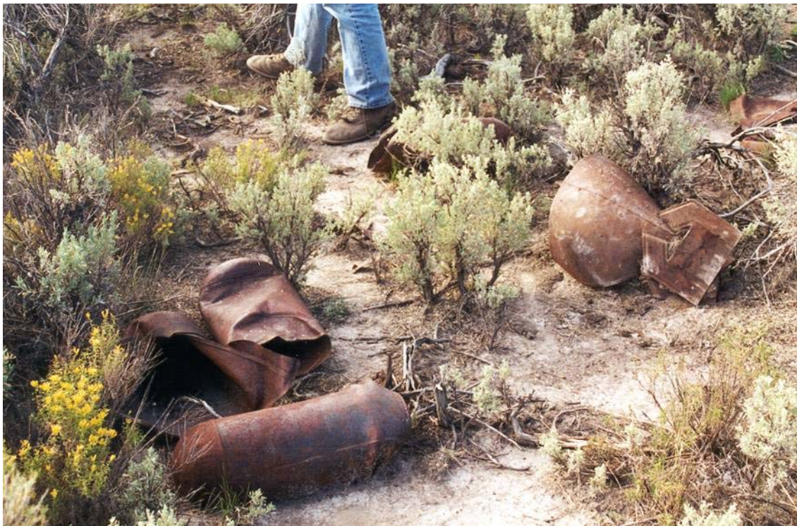
Photo #4 Siskiyou Rocket and Bombing Range – 27-31 August 2001 OE Debris 100-lb. Practice Bombs – nearly complete bodies and tailfins from Navy MK VII or XV.
