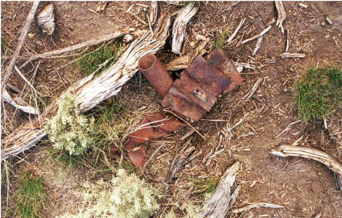
Photo #3 Siskiyou Rocket and Bombing Range – 27-31 August 2001 OE Debris 2.25 inch SCAR (Sub-Caliber Aerial Rocket) – mangled expended rocket motor and fins.
