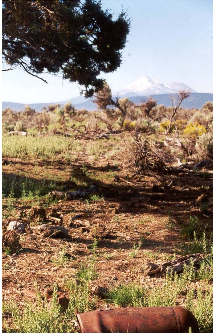
Photo #5 Siskiyou Rocket and Bombing Range – 27-31 August 2001 OE Debris Practice Bomb and Rocket – nearly complete body from 100-lb. Practice Bombs Navy MK VII or XV and mangled expanded rocket motor from 2.25 inch SCAR (Sub-Caliber Aerial Rocket); Mount Shasta in background.
