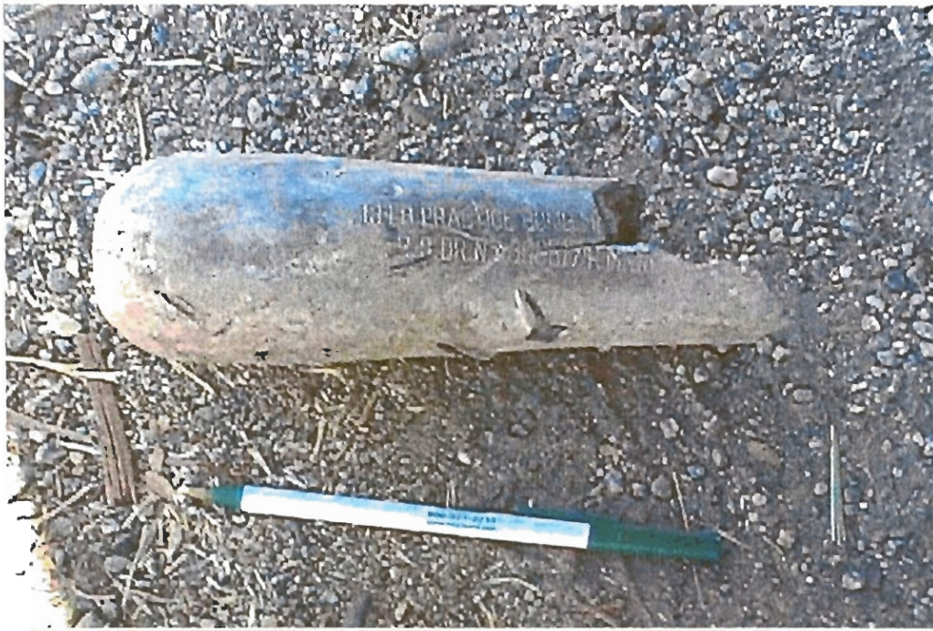
Photo #1 - Hollister 12th Naval District Target No. 5 - 23 August 2001 AN-MK19 Miniature Practice Bomb – Lead antimony bomb found on site by farmer leasing property.
