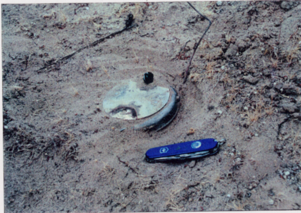
PHOTO #7 LANYARD; TOP DISK IS 3-3/4 " DIAMETER; OVERALL DIAMETER IS 4-1/4"; POSSIBLY FROM AN AIRCRAFT FLARE (LOCATION: N 33°1'52.3" W 115°18'32.2"; PG 57928 55825)
