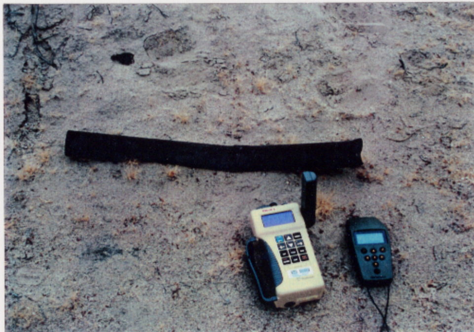
PHOTO #2 2.25" TARGET ROCKET MOTOR, 2.25" DIAMETER, 26" LONG (LOCATION: N 33°1'28.8" W 115°18'31.1"; PG 57967 55102)
