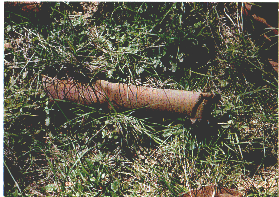
J-4 Area A, 2.25 inch SCAR rocket motor tube in trash pile
