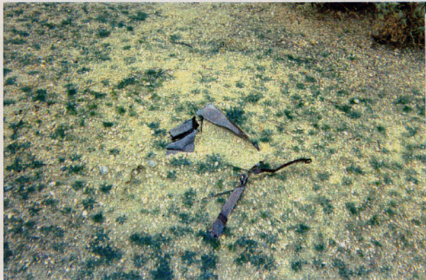
J-9 CRUSHED BODY, SUSPENSION STRAP AND LUG FOR M47 SERIES SAND FILLED BOMB.
