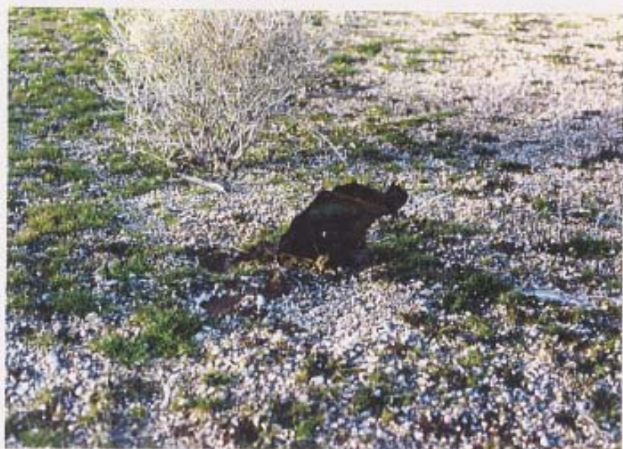
J-12 (Area A) A piece of the tail fin assembly from a M38A2 100-lb. practice bomb. Note the blue coloration still evident on the fin.
