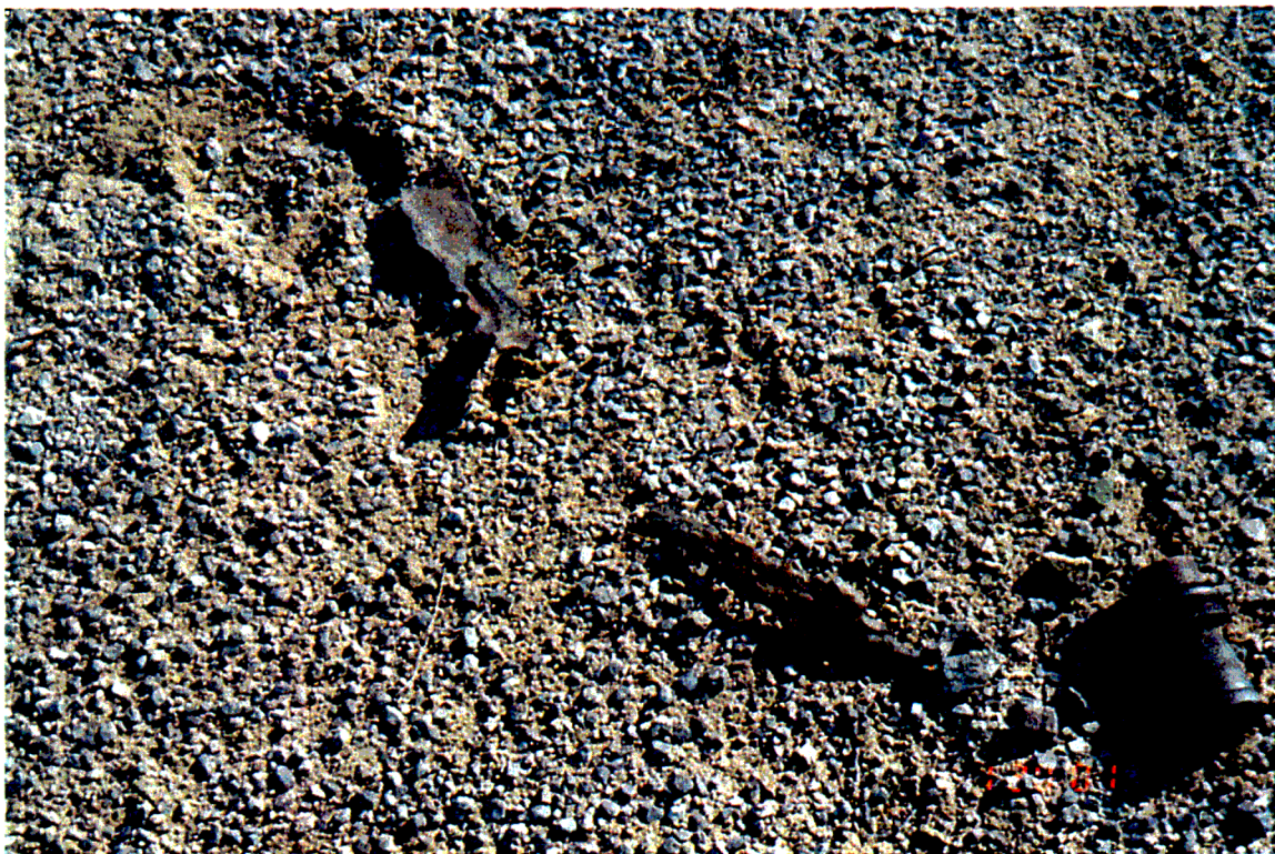
J-18 More shrapnel and part of AN-M100A1 fuze located near a crater west of target. Area "A"
