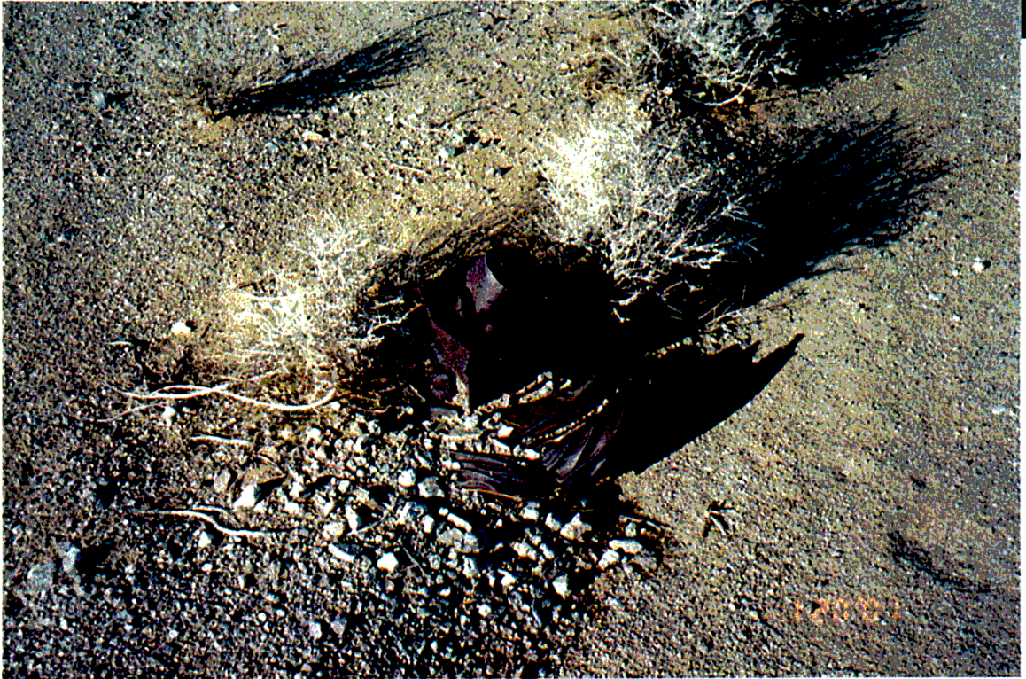
J-11 Impacted M38A2 100 pound practice bomb with an empty M1A1 spotting charge. Found on southern part of section 8. Area "C"
