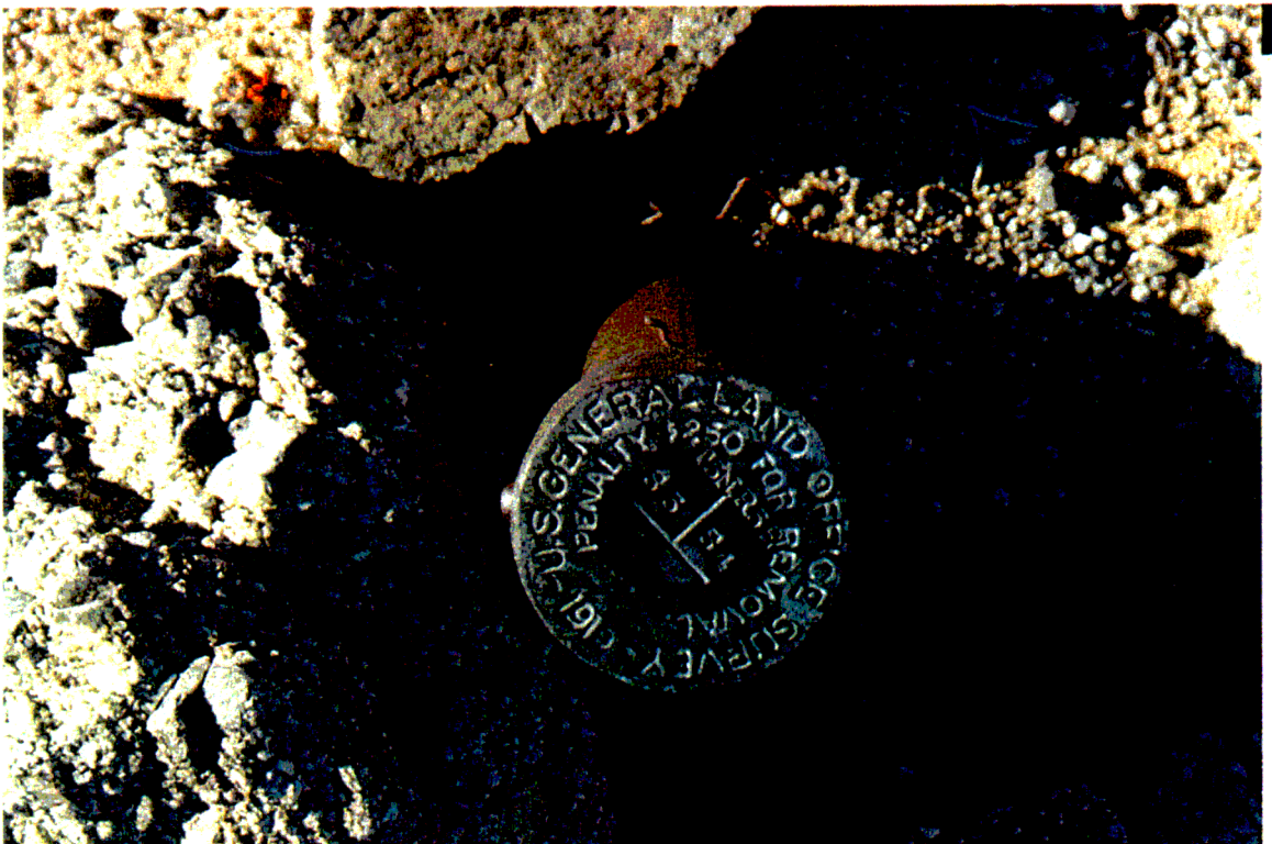
J-12 Survey marker marking the southeast corner of section 5 where target is located. Area "A"
