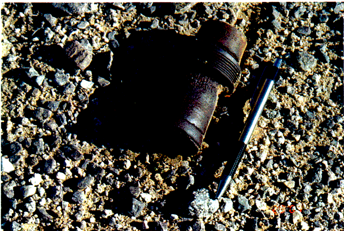
J-16 Part of an AN-M100A1 tail fuze located on north side of target near a crater in section 5. Area "A"
