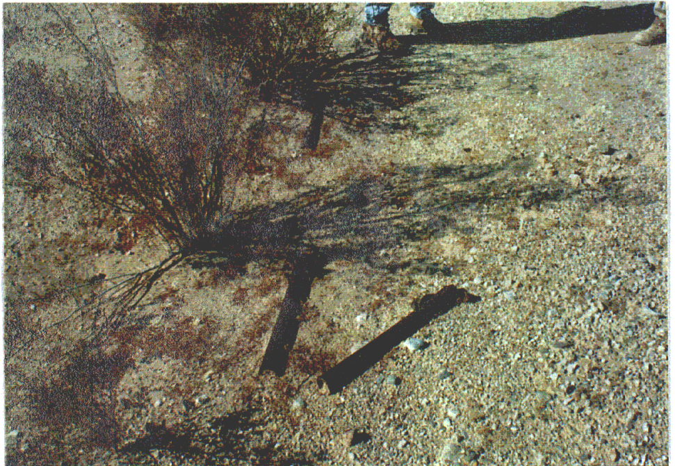
Photo #10 Winona Bombing Target #1 8 February 1996 3.5 inch practice rocket - inert head (steel type)
