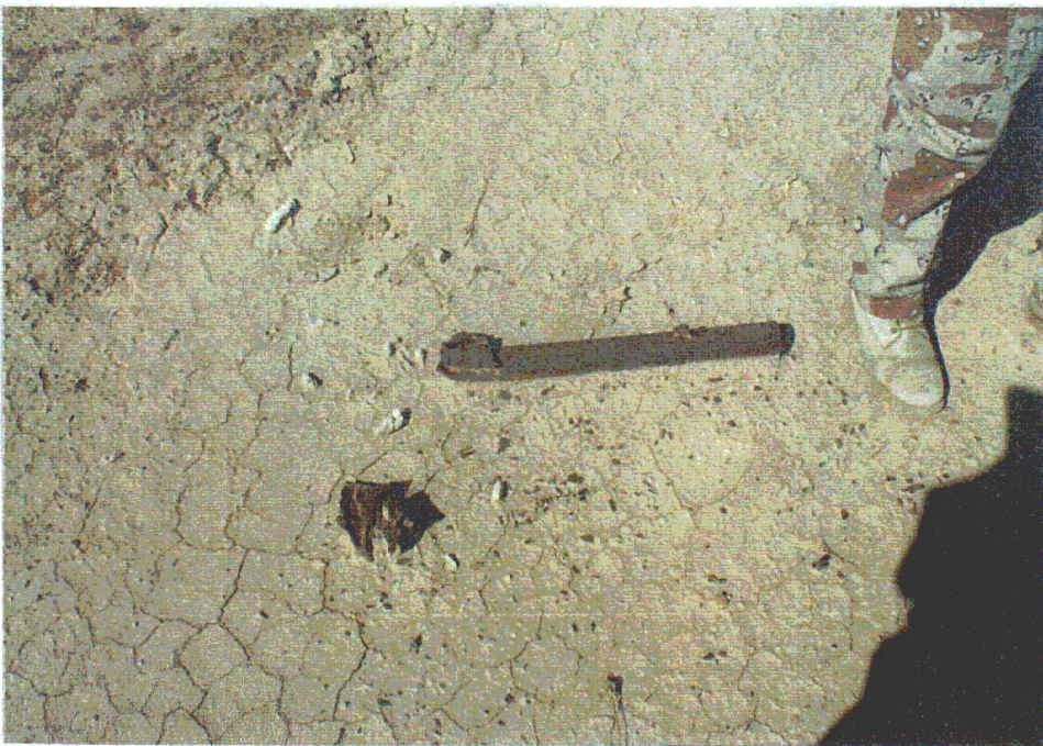
Photo #8 Winona Bombing Target #1 8 February 1996 2.25 inch practice rocket - rocket motor and tailfins
