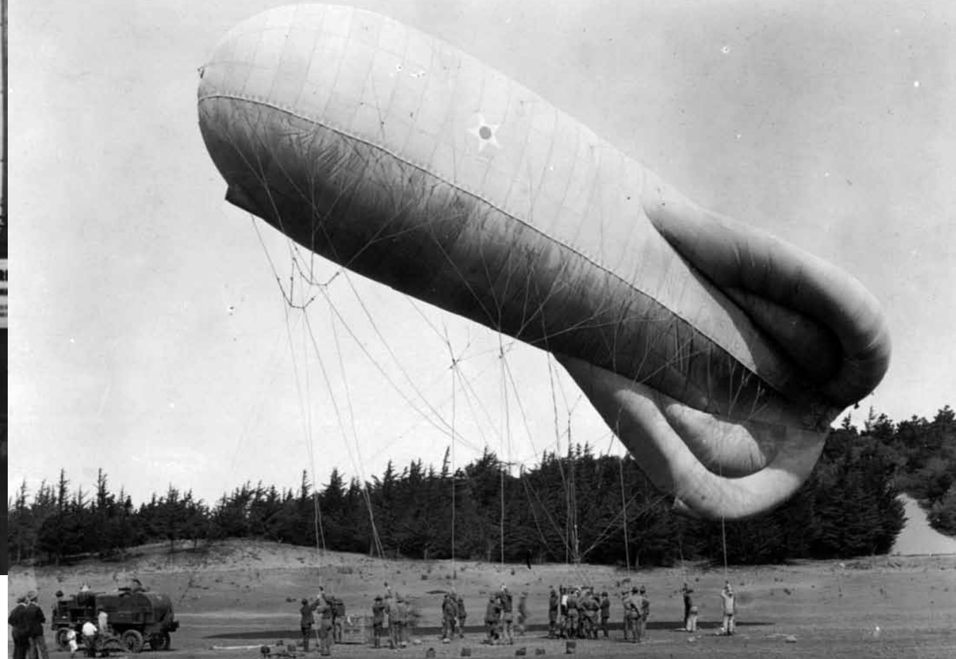
Above: Soldiers preparing their balloon for departure at the Presidio in the 1920s. Measuring 92 ft. long and 32 ft. in diameter, the balloon could stay aloft in winds as high as 70 mph. Dubbed the "sausage balloons," these airships consisted of a hydrogen-filled body with fins that provided stability in rough air and a suspended wicker basket that held a two-man crew. (Photo courtesy of the U.S. Army)
