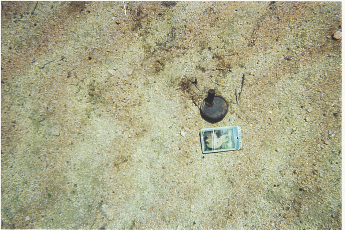
J-5 Remnant of spotting charge used in the M38A2 practice bomb - discovered on surface in Area A.
