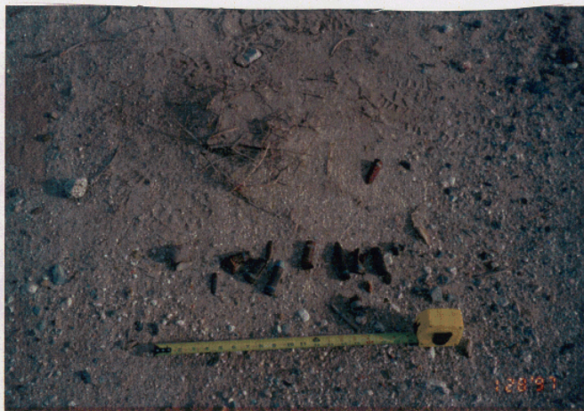
J-13. Area E-1 (Borrego Wash): Assorted M75 20MM Armor Piercing-Tracer Projectiles, M99 20MM Target Practice Projectiles, and .50 Caliber Bullets.
