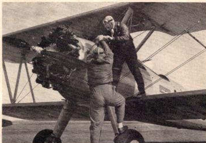
"WINDING 'ER UP" shortly after dawn, the cadets at the right have the trainer's Continental engine almost on the way for the morning's work.
